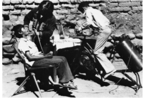
This high-speed dental drill runs on air compressed by bicycle power. It is used by village dental workers in Verano, Mexico.
